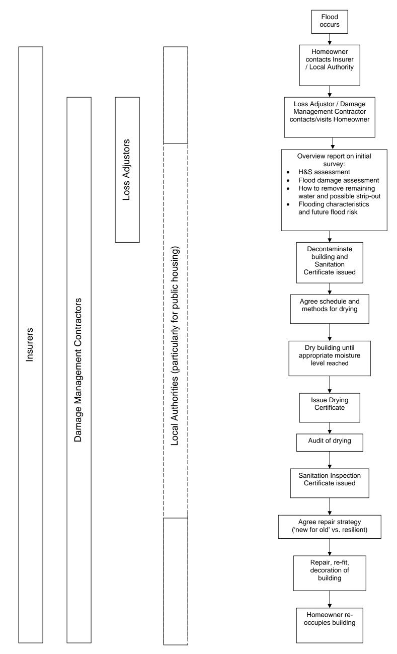
Figure 1.1 Stages in restoration of flooded buildings
