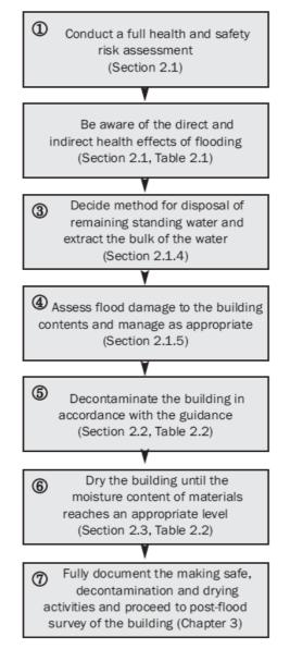
Figure 2.1 Method for safe and effective decontamination and drying of a flooded building
