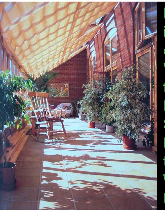
Hot house in the middle of winter Ventilation for summer No heating Solar gain **Exposed** thermal mass Windows and **Doors to house**
