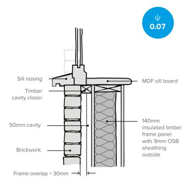
Use a cavity closer with a PU/PIR insulation core to improve performance of sills and jambs.
