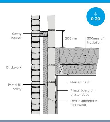
Use lightweight aggregate blockwork on the inner leaf to improve gable performance.
