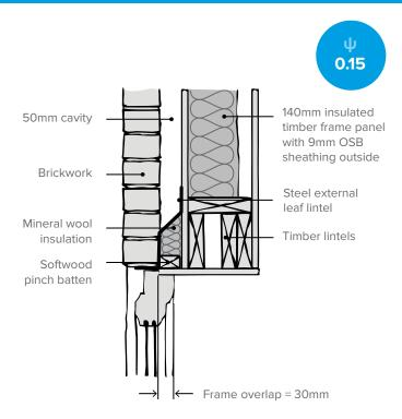
Use an insulated plasterboard reveal to improve performance of timber frame lintels.
