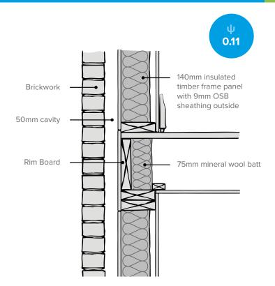
Use an insulated plasterboard on the inside of the frame to improve intermediate floor performance.
