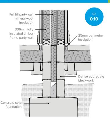
Use lightweight aggregate footing blockwork to improve ground floor performance.
