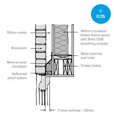
Increase the window frame overlap to improve performance of timber frame lintels.
