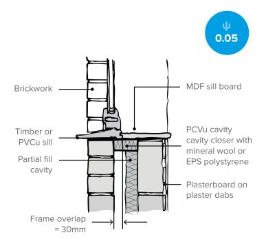
Use a cavity closer with a PU/PIR insulation core to improve the performance of sills and jambs.
