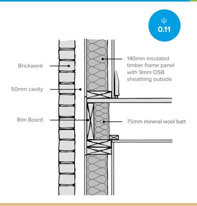
Increase the rimboard insulation thickness to improve intermediate floor performance.
