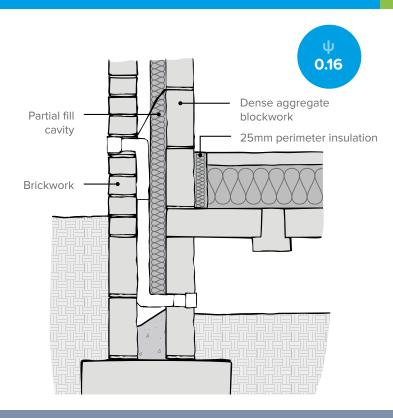
Use lightweight aggregate blockwork on the inner leaf to improve ground floor performance.
